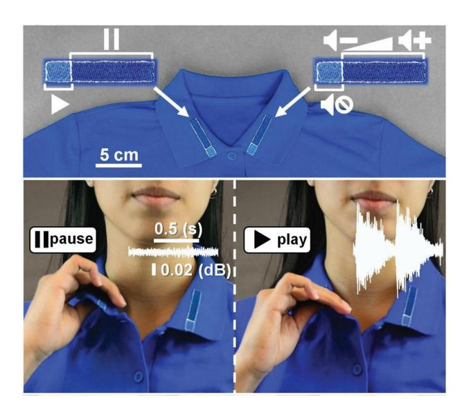
Purdue waterproof, breathable and antibacterial self-powered clothing is based on omniphobic triboelectric nanogenerators. Credit: Ramses Martinez/Purdue University
