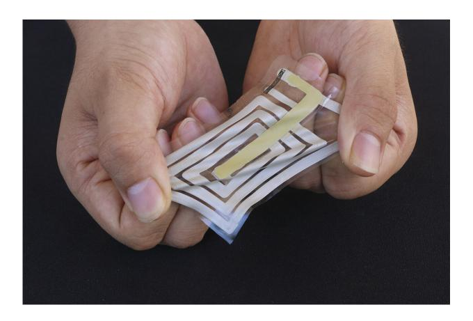
Using metallic ink, researchers screen-print an antenna and sensor onto a stretchable sticker designed to adhere to skin and track pulse and other health indicators, and beam these readings to a receiver on a person's clothing. Credit: Bao Lab
