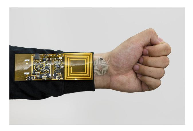
The rubber sticker attached to the wrist can bend and stretch as the person's skin moves, beaming pulse readings to a receiver clipped to the person's clothing. Credit: Bao Lab
