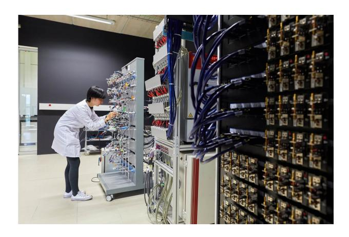
Testing coin cells at battery tester. Credit: CIC energigGUNE
