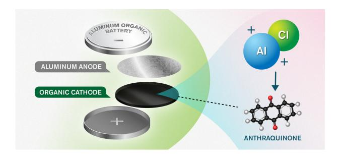
The new concept consists of an anode and cathode made of aluminium and an anthraquinone-based organic material, respectively. The organic cathode material enables efficient storage of the positive charge carriers from an aluminium and chlorine-based electrolyte - the solution in which ions can move between the electrodes. Credit: Yen Strandqvist/Chalmers University of Technology
