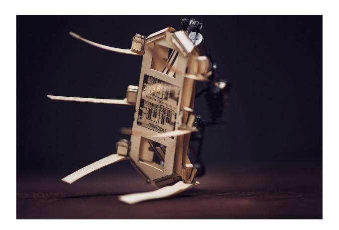
A prototype demonstrates the circuitry and manufacturing technology being developed for a robotic pill that could give farmers an inside view of the health of each cow by moving among their stomach chambers. Credit: Purdue University photo/Rebecca Wilcox
