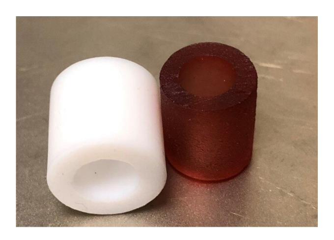
Photograph of PTFE (left) and HIPEP (right) propellant samples used in the test. Credit: University of Illinois Department of Aerospace Engineering
