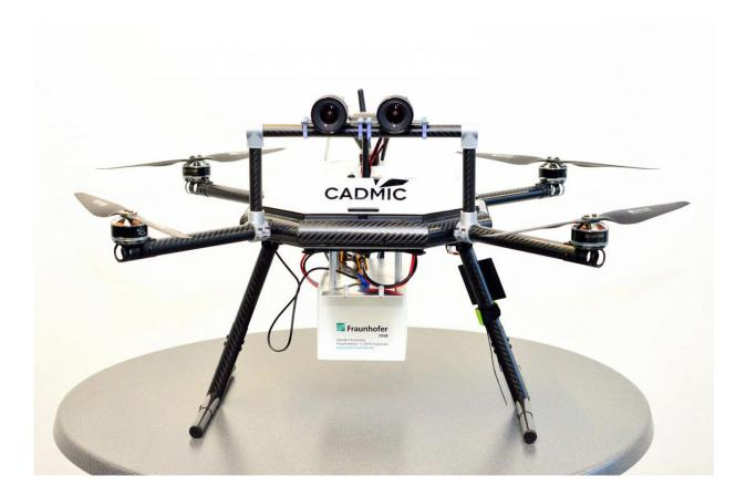
Drone with stereo camera. The small white box holds the embedded system, which evaluates the slightly offset images from the two cameras in real time in order to detect obstacles. Credit: Fraunhofer IOSB
