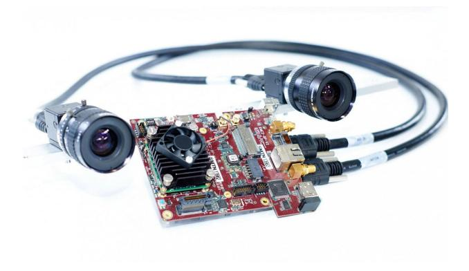
The stereo camera and the embedded system installed on the drone. Credit: Fraunhofer IOSB
