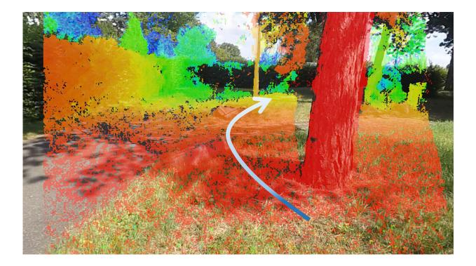
The same image with overlaid depth information from the stereo image analysis, highlighting close obstacles in red. The arrow indicates the resulting recommended evasive path. Credit: Fraunhofer IOSB
