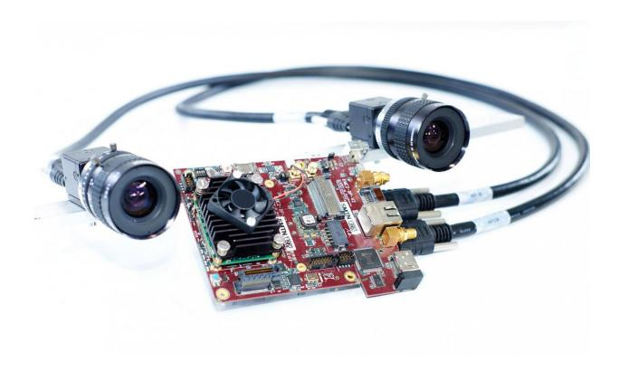
The stereo camera and the embedded system installed on the drone. Credit: Fraunhofer IOSB
