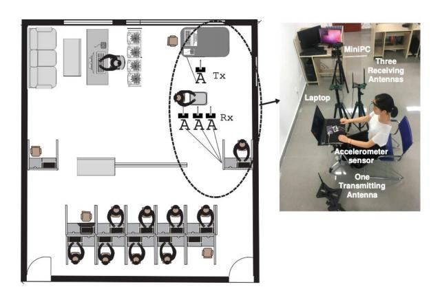
The prototype emotion sensing system developed by the researchers. Credit: Gu et al.
