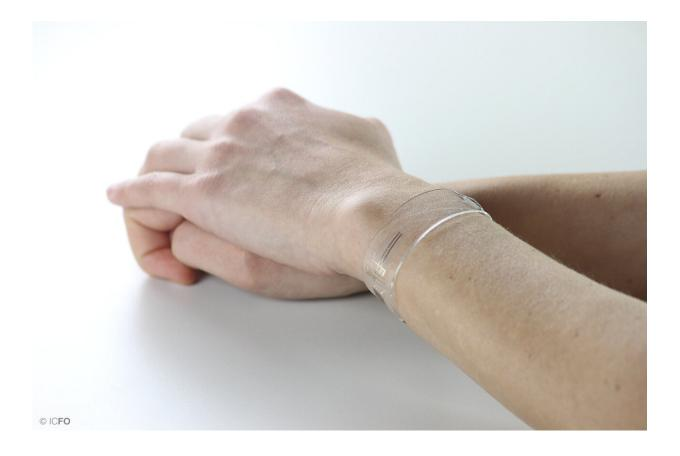
Flexible and transparent bracelet that uses graphene to measure heart rate, respiration rate and blood pulse oxygenation continuously. Credit: ICFO
