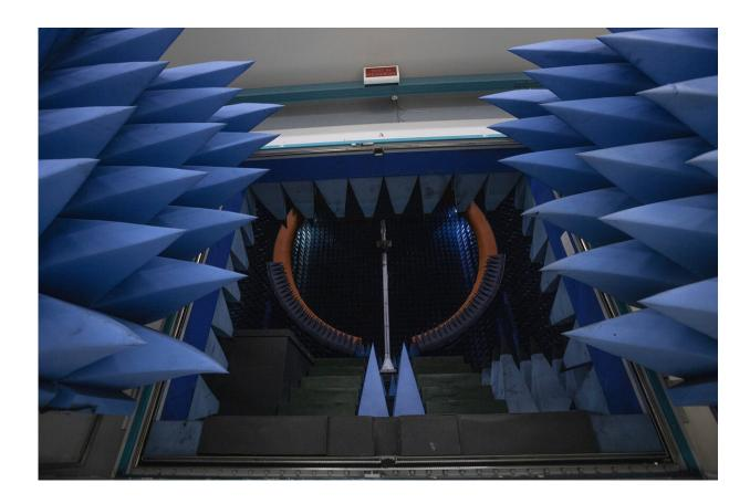
In this Aug. 21, 2019, photo, doors lead to the Spherical Near Field Test System used for testing antennas at the Huawei lab in Dongguan in Southern China's Guangdong province. Facing a ban on access to U.S. technology, Chinese telecom equipment maker Huawei is showing it increasingly can do without American components and compete with Western industry leaders in pioneering research. (AP Photo/Ng Han Guan)
