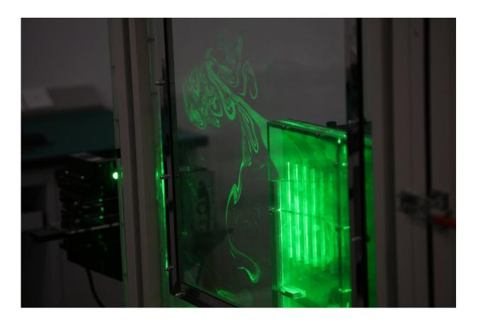
In this Aug. 21, 2019, photo, lasers are used to demonstrate heat flow from heat sink designs at the Huawei Thermal design lab in Dongguan in Southern China's Guangdong province. Facing a ban on access to U.S. technology, Chinese telecom equipment maker Huawei is showing it increasingly can do without American components and compete with Western industry leaders in pioneering research. (AP Photo/Ng Han Guan)
