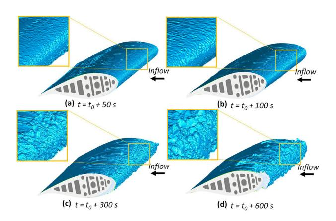
This image from experiments in Iowa State's Icing Research Tunnel show the evolution of icing on a model wind turbine blade, with glaze ice growing rougher and rougher at 50, 100, 300 and 600 seconds. Larger image. Credit: Hui Hu.
