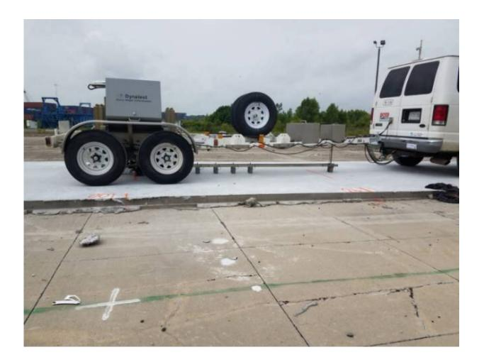
LSU researchers constructed three 60-foot-long overlay sections on top of a section of deteriorated asphalt at the Louisiana Transportation Research Center in order to restore its condition. Credit: LSU College of Engineering
