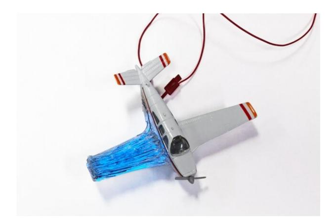
Using the 3-D printing method developed by the MIT researchers, a structure such as this model airplane wing could have both light emitters and light detectors embedded in the material, so that it could continuously detect any micro-cracks as they begin to form. Credit: Felice Frankel
