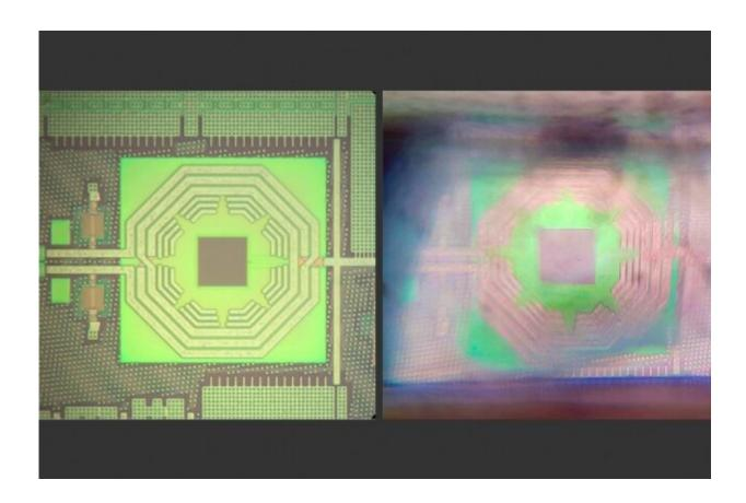
MIT researchers have fabricated a diamond-based quantum sensor on a silicon chip using traditional fabrication techniques (pictured), which could enable lowcost quantum hardware. Credit: Massachusetts Institute of Technology
