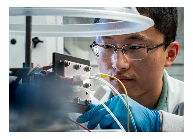
Rice University engineer Haotian Wang adjusts the electrocatalysis reactor built in his lab to recycle carbon dioxide to produce liquid fuel. The reactor is designed to be an efficient and profitable way to reuse the greenhouse gas and keep it out of the atmosphere. Credit: Jeff Fitlow/Rice University
