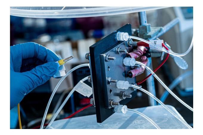
An electrocatalysis reactor built at Rice University recycles carbon dioxide to produce pure liquid fuel solutions using electricity. The scientists behind the invention hope it will become an efficient and profitable way to reuse the greenhouse gas and keep it out of the atmosphere. Credit: Jeff Fitlow/Rice University
