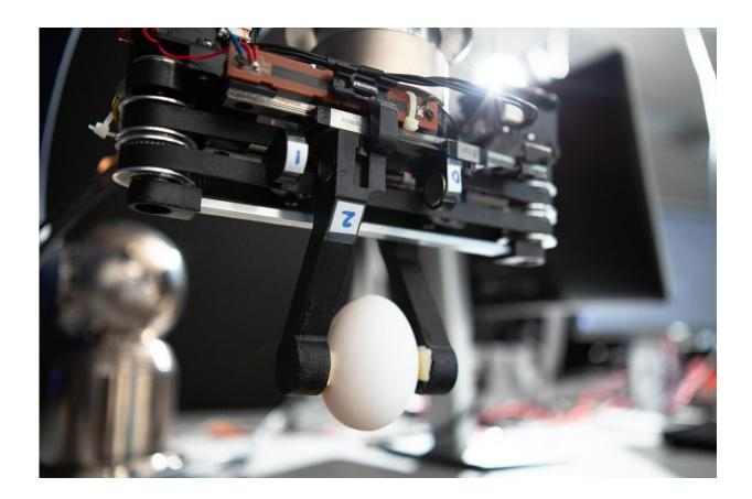
A robotic gripper developed in the lab of University at Buffalo engineer Ehsan Esfahani uses repulsion between magnets to adjust the stiffness of its grip, improving safety. Credit: Douglas Levere/University at Buffalo
