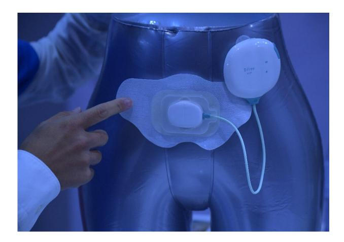
High-tech relief for the incontinent is offered by D-Free, a sensor which fits on the abdomen and detects changes in bladder size
