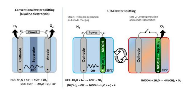
Image showing the difference between the conventional approach to water splitting (alkaline electrolysis) and the E-TAC water splitting technique proposed by the researchers. Credit: Dotan et al.
