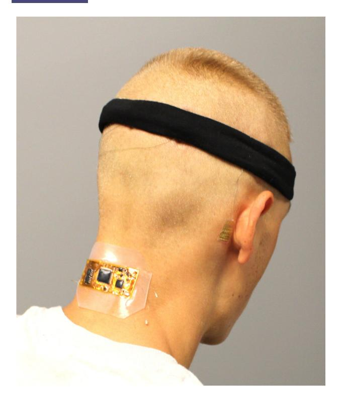
Test subject who has flexible wireless electronics conformed to the back of the neck, with dry hair electrodes under a fabric headband and a membrane electrode on the mastoid, connected with thin-film cables. Credit: Woon-Hong Yeo
