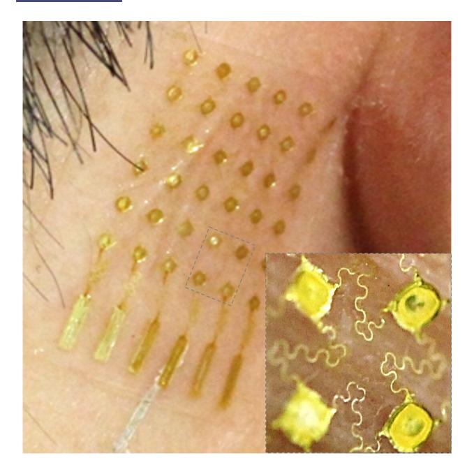
An aerosol-jet printed stretchable, skin-like electrode with an open-mesh structure shown in inset. Credit: Woon-Hong Yeo
