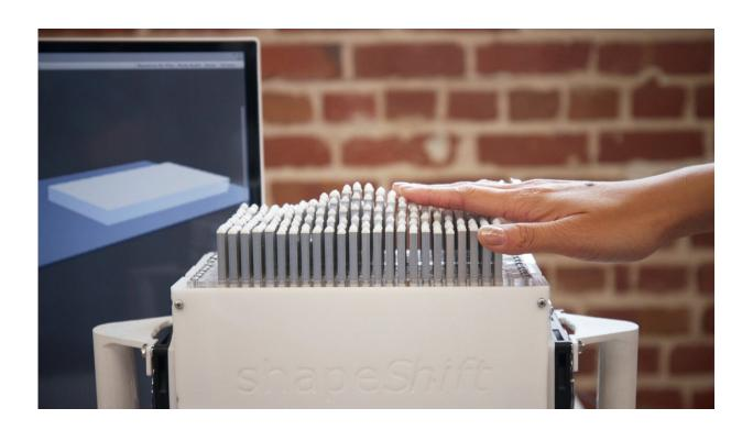
The display is reminiscent of a pin art toy in that it forms shapes from a field of tall, rectangular pegs that move up and down. Credit: Farrin Abbott
