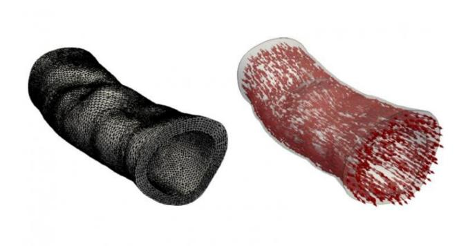
These arterial models were created from a patient-specific scan. The model on the left is the fundamental 'mesh' required to split the artery into many pieces to model the stresses within. The figure on the right is modeling how a material property is propagated through the artery in a single direction. Credit: Duke University
