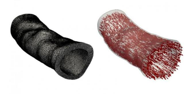
These arterial models were created from a patient-specific scan. The model on the left is the fundamental 'mesh' required to split the artery into many pieces to model the stresses within. The figure on the right is modeling how a material property is propagated through the artery in a single direction. Credit: Duke University
