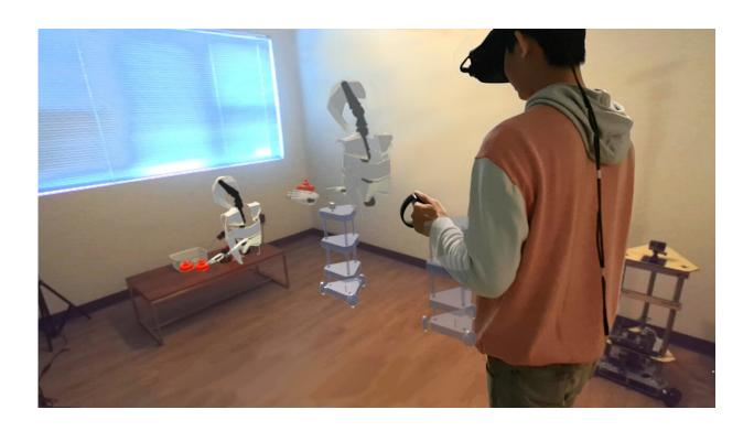
A new augmented reality platform, GhostX, uses 'ghost' avatars of a human and robot to help a user plan out how the two can perform a task together. Credit: Purdue University image/Yuanzhi Cao
