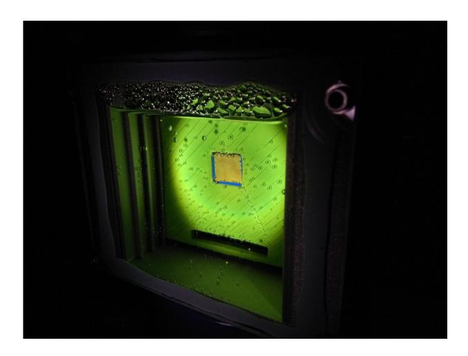
This 'artificial leaf' uses water, sunlight and carbon dioxide to produce a widelyused gas, inspired by the natural process by which plants use the energy from sunlight to turn carbon dioxide into food. Credit: Virgil Andrei
