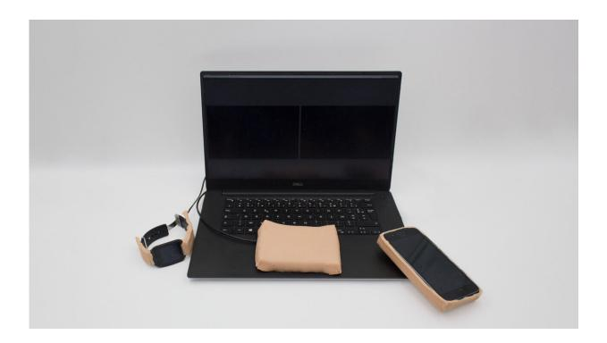
A new interface developed by researchers in Bristol and Paris takes touch technology to the next level by providing an artificial skin-like membrane for augmenting interactive devices such as phones, wearables or computers. Credit: Marc Teyssier
