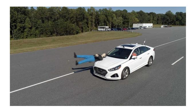
The 2019 Hyundai Sonata received "no credit" from the Insurance Institute for Highway Safety when its automatic emergency braking system failed to prevent the car from crashing into this pedestrian dummy. Credit: IIHS
