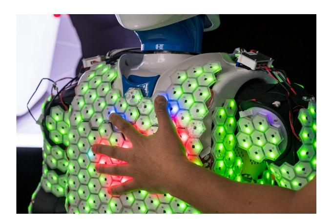
Each cell of this artificial skin developed by researchers at the Technical University of Munich (TUM) is equipped with a microprocessor and sensors to detect contact, acceleration, proximity and temperature. New control algorithms made it possible for the first time to apply artificial skin to a human-sized robot. Credit: Astrid Eckert/TUM
