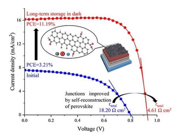
The initial power conversion efficiency (PCE) soared after long-term storage because of the self-recrystallization process that perovskite undergoes when stored in the dark. Much higher conductivity and lower resistance was observed for perovskite covered with carbon nanotubes (CNTs) with oxygen-containing functional groups. Credit: Tokyo Tech
