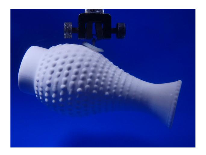
The suction cup researchers developed is capable of lifting bumpy objects. It also lifts many times its weight in and out of water. Credit: University of California San Diego
