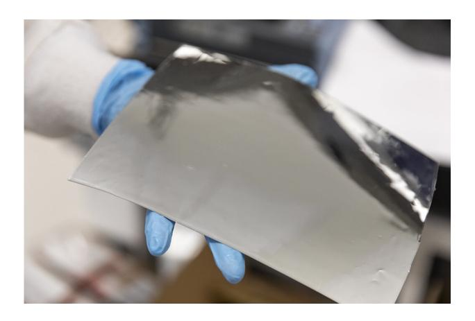
The PDMS/aluminum film manufactured by the team in the lab. Credit: KAUST
