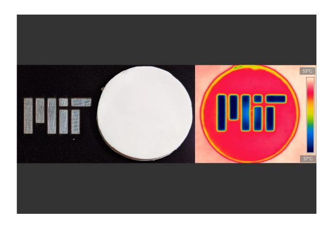
In the photo on the left, a disk of the new insulating material blocks and reflects visible light, hiding the MIT logo beneath it. But seen in infrared light, at right, the material is transparent and the logo is visible. Credit: Arny Leroy, Evelyn Wang, et. al
