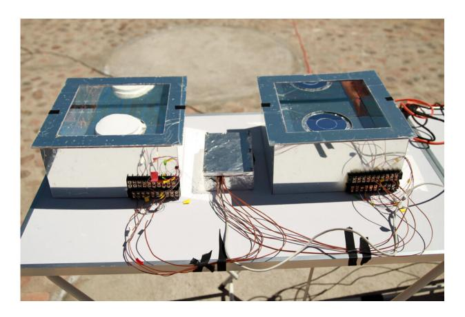
In field tests, the performance of the radiative cooling device was measured under full sunlight, both with the insulating material in place (left) and without it (right). Credit: Massachusetts Institute of Technology
