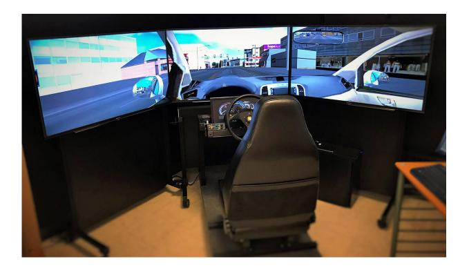
Experiments using this driving simulation will help researchers to develop algorithms that allow an autonomous vehicle to understand and predict human behavior. Credit: Purdue University photo/DeEtte Starr
