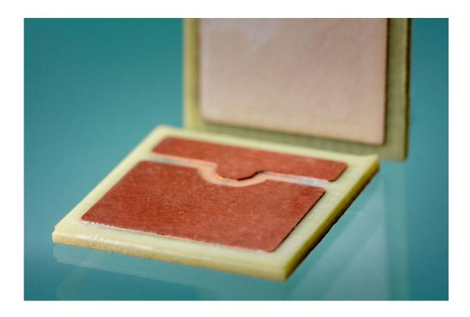
Embedded silicon carbide on its way to mass manufacturing for e-mobility applications. Credit: Volker Mai/Fraunhofer IZM
