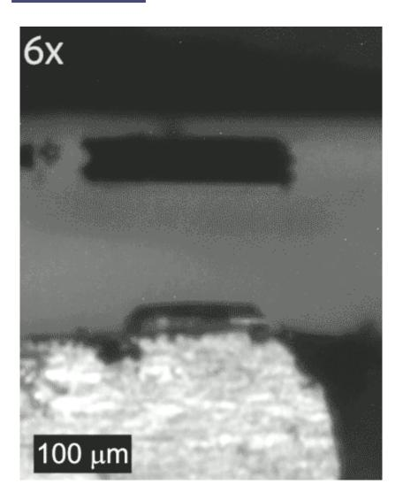
New electroadhesive stamp picks and places a 170-micrometer sized LED chiplet, using an external voltage of 30V to temporarily "stick" to the LED. Credit: Courtesy of the researchers
