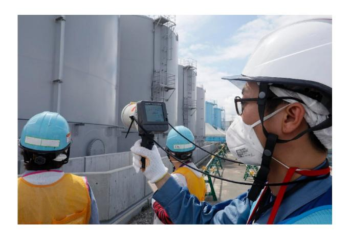
Staff measure radiation levels around the storage tanks of radiation-contaminated water at the tsunami-crippled Tokyo Electric Power Company (TEPCO) Fukushima Dai-ichi nuclear power plant in Japan
