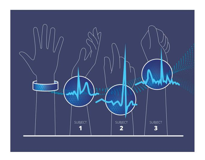
Sandia National Laboratories is testing biometric technology that uses unique electrocardiogram signals sent from a wearable device, possibly a wristband or chest strap, to identify a person for security purposes. Credit: Michael Vittitow, Sandia National Laboratories
