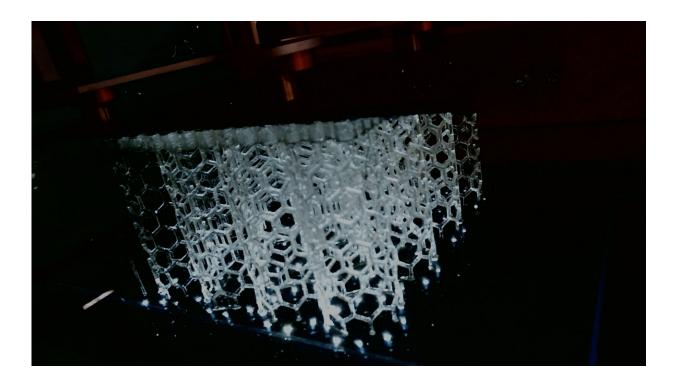
High-area rapid printing technology prints vertically, using ultraviolet light to cure liquid resin into hardened plastic. Credit: Northwestern University
