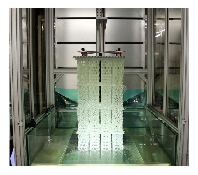
At 13-feet tall and with a 2.5-feet wide print bed, HARP is the biggest 3D printer to date. Its size allows it to print large, continuous structure or many, different small structures at once. Credit: Northwestern University
