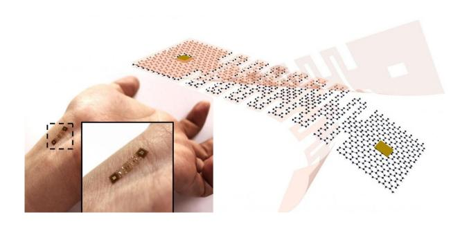
Using kirigami to cut and fold graphene allows wearable sensors to better conform with the natural movement of the body. Credit: University of Illinois at Urbana-Champaign Department of Mechanical Science and Engineering.
