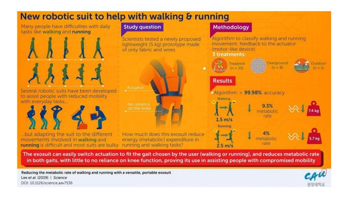
Newly developed robot suit made of fabric vest and wires will help people with restricted mobility to walk and run more efficiently. Credit: Chung-Ang University
