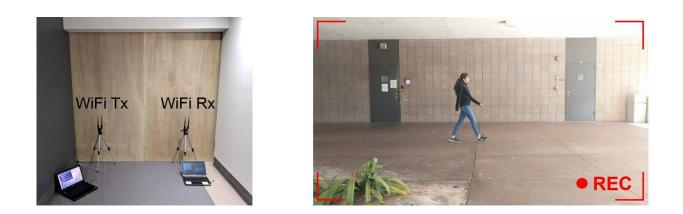
(left) A pair of WiFi transceivers are inserted outside. The transmitter sends a wireless signal whose received power (or magnitude) is measured by the receiver. Then, given the video footage on the right — and by using only such received power measurements — XModal-ID can determine if the person behind the wall of the left figure is the same person in the video footage. Credit: B. Korany et al.
