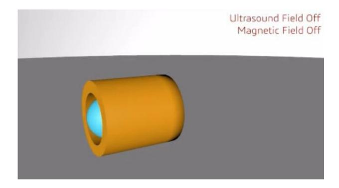
A new type of micromotor—powered by ultrasound and steered by magnets—can move around individual cells and microscopic particles in crowded environments without damaging them. The technology could open up new possibilities for targeted drug delivery, nanomedicine, tissue engineering, regenerative medicine and other biomedical applications.
