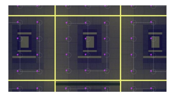
An analog circuit solves combinatorial optimization problems by using oscillators' natural tendency to synchronize. The technology could scale up to solve these problems faster than digital computers. Credit: Bryan Mastergeorge
