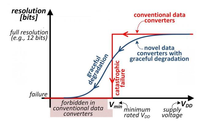
Catastrophic failure is replaced by graceful resolution degradation in the novel class of conventional data converters invented by the NUS team. This allows to drastically simplify the system design, suppressing the need for accurate voltage regulation. Credit: National University of Singapore
