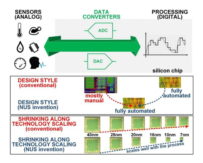
Catastrophic failure is replaced by graceful resolution degradation in the novel class of conventional data converters invented by the NUS researchers. Credit: National University of Singapore
