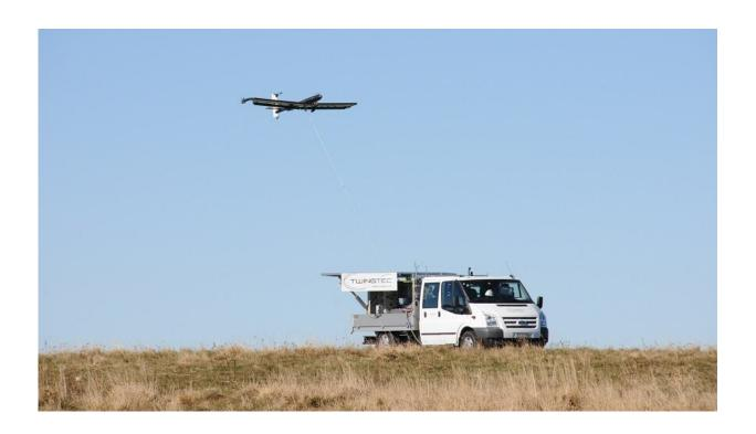
Successful test flight on the heights of the Chasseral in autumn 2018: TwingTec prototype T 28, a device with a wing-span of three meters, took off independently from its base vehicle, climbed into the air, circled autonomously in the air for 30 minutes, produced electrical energy and finally landed safely again on the launch platform. Credit: Empa
