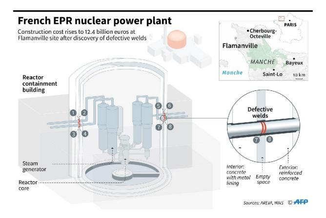
Graphic of the EPR nuclear power plant under construction at Flamanville in France, locating defective welds which had led to a new cost blowout to 12.4 billion euros.
