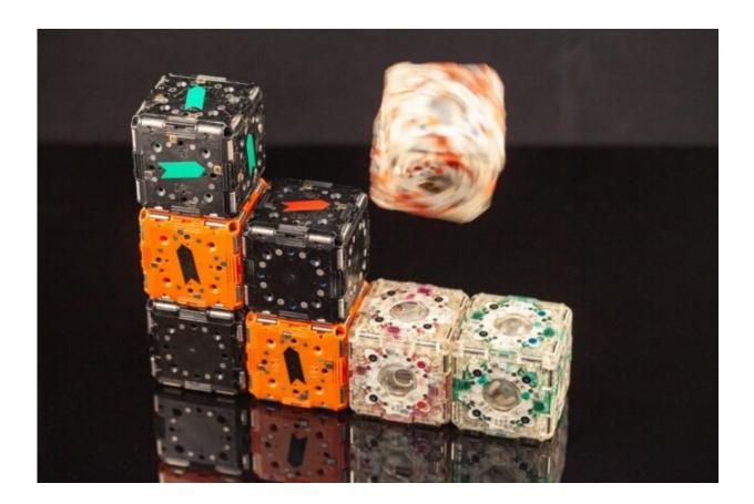
One modular robotic cube snaps into place with rest of the M-blocks. Credit: Jason Dorfman/MIT CSAIL
