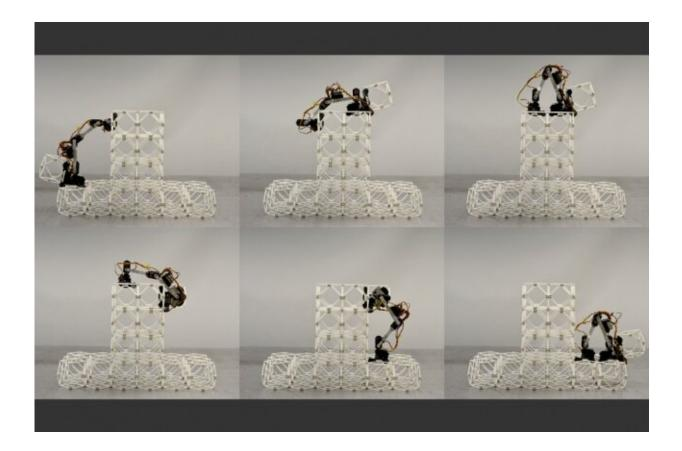
Sequence of photos shows an assembler robot at work, carrying one structural unit over the top and down the other side of a structure under construction. Credit: Benjamin Jenett
