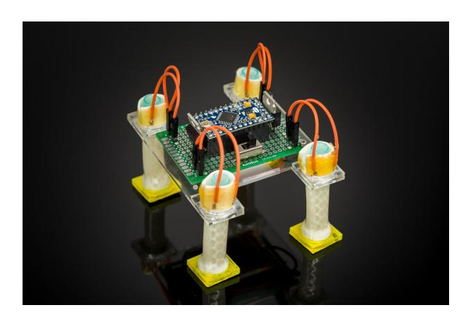
Electrically controlled, untethered soft robot built out of four soft tubular actuators, a microcontroller and battery. The robot can be programmed to walk or carry an object. Credit: David Baillot/UC San Diego Jacobs School of Engineering
