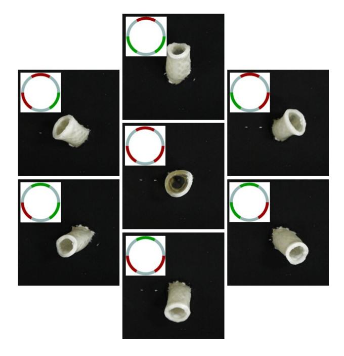
Depending on which heating wires are electrically activated (red), the soft tubular actuator can bend in six different directions (outer images) and contract in length (center image). Credit: Qiguang He
