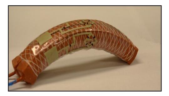
Researchers have devised a soft neurorobot with a neurologically integrated tactile sensory skin, allowing it to sense interactions with the external environment and respond accordingly. Credit: University of Houston
