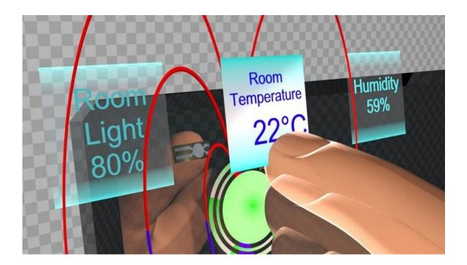
An international research team has developed an electronic sensor, which can process touchless as well as tactile signals. This "electronic skin" could provide a better interface between humans and machines. Credit: HZDR/D. Makarov
