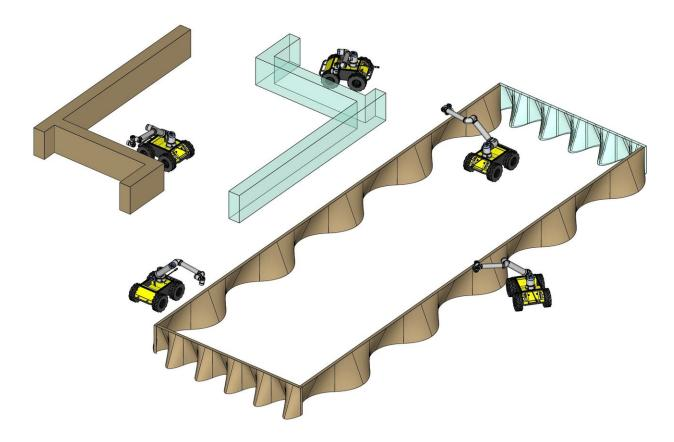
NYU Tandon professors Chen Feng, Ludovic Righetti and Maurizio Porfiri are designing systems for collective additive manufacturing, in which teams of mobile 3D-printing robots work together to repair or build structures, or even work on the moon or Mars. Credit: NYU Tandon
